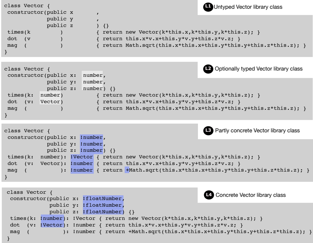
■ Figure 1 Gradual insertion of type annotations to a Vector class in StrongScript.
