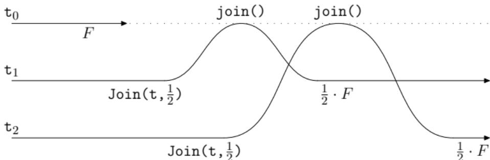
Threads  $t_1$  and  $t_2$  both take back half of  $t_0$ 's resource.
