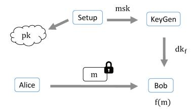
Figure 1.2: Illustration of Functional Encryption. In this scenario, the setup generates a public key pk that Alice uses to encrypt the message m, and sends the ciphertext to Bob. The setup also generates a master secret key msk, that is used by a key generation algorithm to generate a functional decryption key  $dk_f$  associated with the function f. Upon receiving this decryption key, Bob recovers the value f(m) from the encryption of m.
