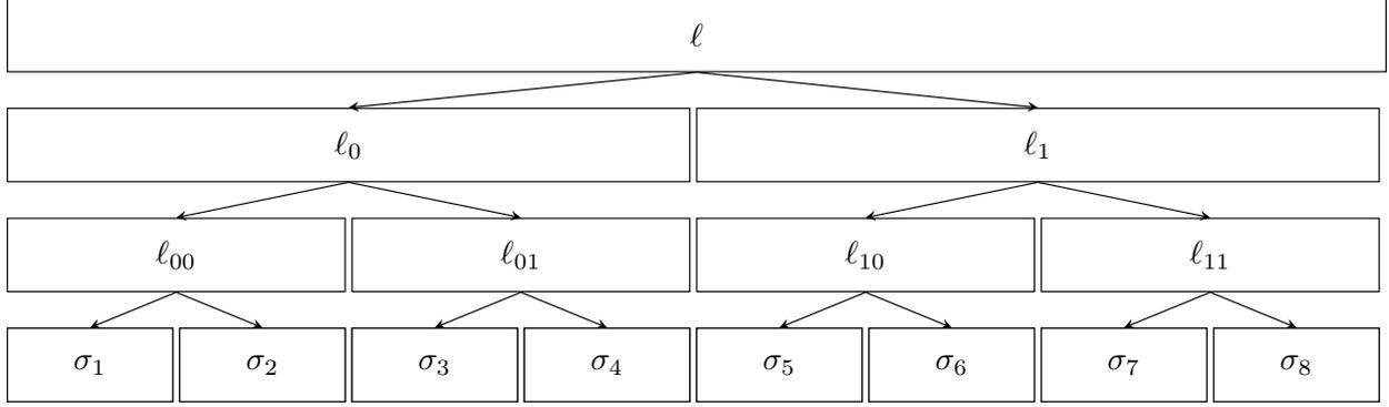
Figure 3.1: A FALCON binary tree of height 3
