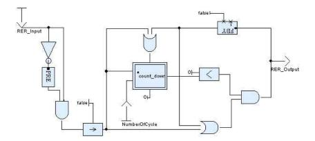
Figure 1.2: A classical operator in SCADE/LUSTRE
