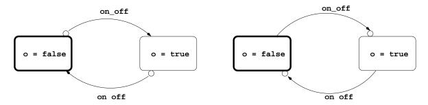
Figure 1.5: Two automata with strong and weak transitions
