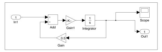
Figure 2: A SIMULINK block-diagram
