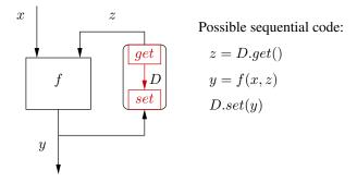
Figure 4: The get/set principle breaks feedback loops
