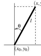
Figure 8: The Inverted Pendulum
