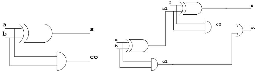
Figure 3: Hierarchical definition of a 1-bit adder
