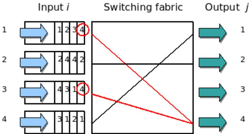
(b) In the Virtual Output Queues (VOQ) architecture, a separate queue is maintained for each output port at each input port. Explain why it solves the HOL blocking problem.
