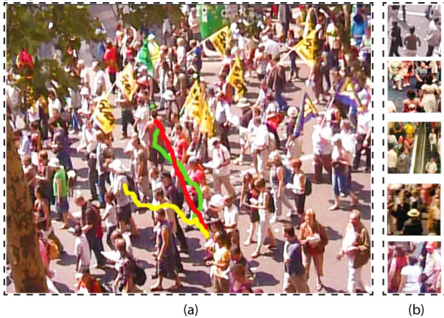
Figure 10. (a) Data-driven track of a person walking across a crowded demonstration (green), ground-truth (red), batch mode tracking (yellow). (b) Matching crowd patches from the database.
