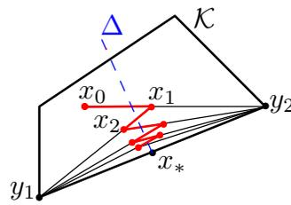
**Figure 4.** Frank–Wolfe algorithm zigzagging. Starting from  $x_0$ , the algorithm always moves toward one of the extreme points of  $\mathcal{K}$  with an average direction of  $\Delta$ .
