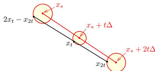
**Figure 1.** Illustration of Richardson extrapolation for  $t_\infty = 0$  and  $x_t = x_* + t\Delta + O(t^2)$ . Iterates (in black) with their first-order expansions (in red). The deviations (represented by circles) are of order  $O(t^2)$ . Adapted from [22].
