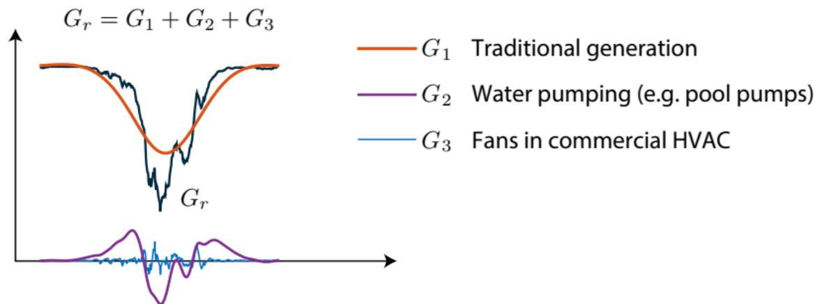
**Demand Dispatch:** Power consumption from loads varies automatically and continuously to provide service to the grid, without impacting QoS to the consumer
