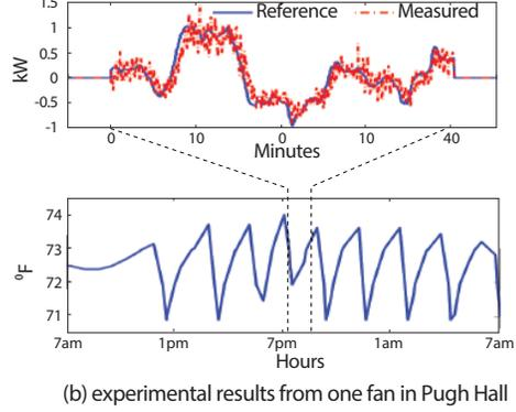
Figure 5: VSFL from a single HVAC fan in a commercial building.
