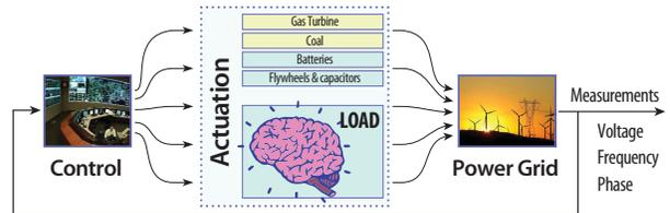
Figure 3: Power grid as a feedback control system.
