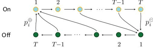
Figure 6: State transition diagram for the pool-pump model.
