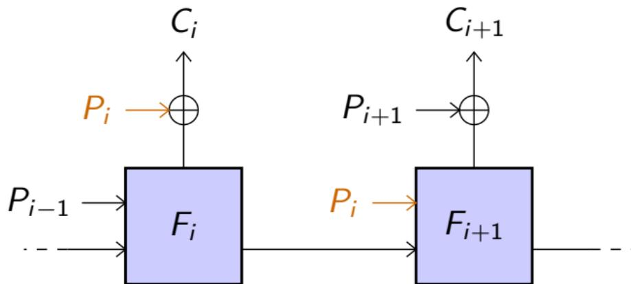
$P_i$  is inserted into the state after  $C_i$  is output.
