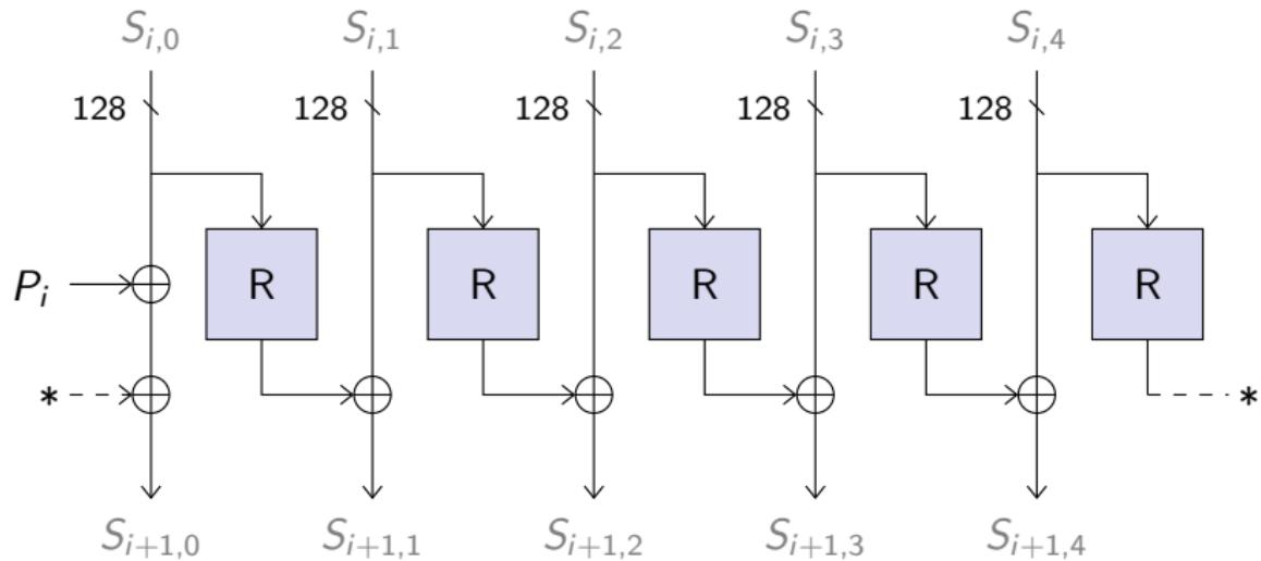
Inner state :  $5 \times 128$  bits in registers  $S_{i,0}, \dots, S_{i,4}$ .
