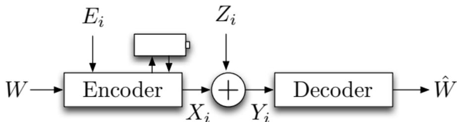
Figure: EH communication system block diagram
