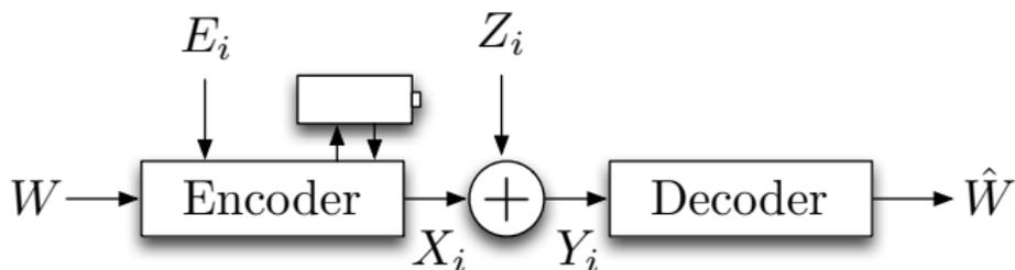
Figure: EH communication system block diagram
