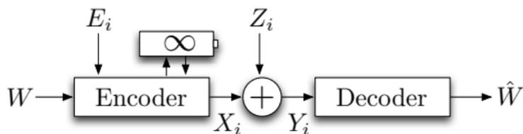
Figure: Infinite battery EH transmitter
