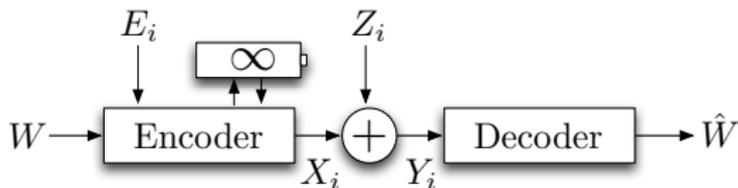
Figure: Infinite battery EH transmitter
