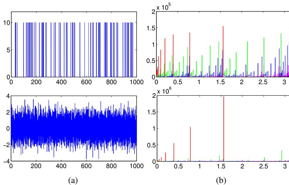
FIGURE 4.2. (a) Realization of a Bernoulli process  $X_1(x)$  at the top and a Gaussian white noise  $X_2(x)$  at the bottom, both having a unit variance. (b) Scattering power spectrum  $PX_i(q(\omega))$  of each process as a function of  $\omega \in [0, \pi]$ . The values of  $PX_i(q(\omega))$  are displayed in red, green, blue, and violet for paths  $q(\omega)$  of lengths 1, 2, 3, and 4, respectively.
