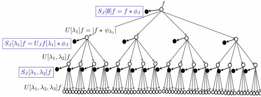
FIGURE 2.1. A scattering propagator  $U_J$  applied to  $f$  computes each  $U[\lambda_1]f = |f \star \psi_{\lambda_1}|$  and outputs  $S_J[\emptyset]f = f \star \phi_{2^J}$ . Applying  $U_J$  to each  $U[\lambda_1]f$  computes all  $U[\lambda_1, \lambda_2]f$  and outputs  $S_J[\lambda_1] = U[\lambda_1] \star \phi_{2^J}$ . Applying iteratively  $U_J$  to each  $U[p]f$  outputs  $S_J[p]f = U[p]f \star \phi_{2^J}$  and computes the next path layer.
