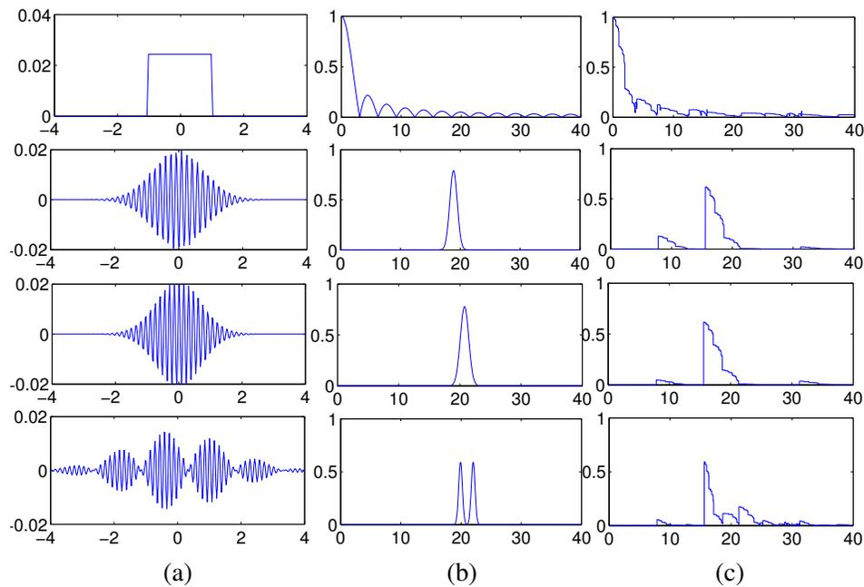
FIGURE 3.2. (a) Each row  $1 \leq i \leq 4$  gives an example of function  $f_i(x)$ . (b) Graphs of the Fourier modulus  $|\hat{f}_i(\omega)|$  as a function of  $\omega$ . (c) Graphs of the scattering  $\bar{S} f_i(q(\omega))$  as a function of  $\omega$ .
