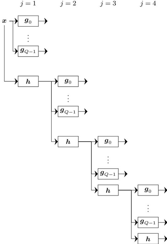
Fig. 3: Multirate filter bank computing wavelet coefficients for  $J = 4$ . Each block corresponds to a filter convolution subsampled by 2 where a boxed  $h$  is a low-pass filter and a boxed  $g_k$  is a band-pass filter. The depth corresponds to the octave index  $j$  while  $k = 0, \dots, Q - 1$  is the suboctave index.
