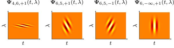
Fig. 7: Real parts of four time-frequency wavelets  $\Psi_{\mu,\ell,s}(t, \lambda)$ .
