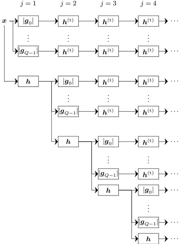
Fig. 4: Mel-spectrogram implemented as a convolutional network. Each  $|g_k|$  block convolves by a band-pass filter  $g_k[n]$ , computes the modulus, and subsamples by 2. Blocks containing  $h$  or  $h^{(t)}$  convolve by a low-pass filter and subsample by 2.
