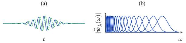
Fig. 2: (a) Real and imaginary parts of a Morlet mother wavelet with  $Q = 4$ . (b) The resulting wavelet filter bank in Fourier.
