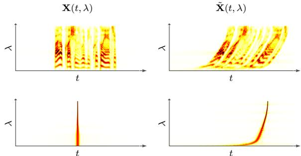
Fig. 6: Effect of frequency-dependent time-shifts  $\tau(\lambda)$  on scalograms of a speech recording (top) and a Dirac delta function (bottom). The two columns correspond to the original signal  $x(t)$  and the transformed signal  $\tilde{x}(t)$ , respectively.
