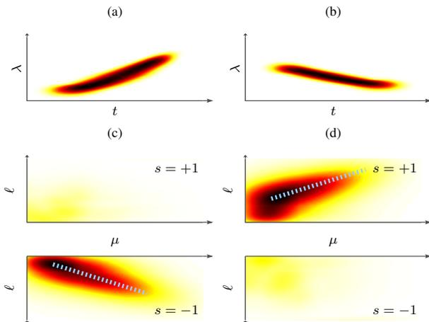
Fig. 9: Scalograms of two exponential chirps with chirp rates (a)  $\alpha = 4$  and (b)  $\alpha = -2$ . (c, d) Corresponding second-order joint time-frequency scattering coefficients  $\mathbf{S}_2\mathbf{x}(t, \lambda, \mu, \ell, s)$  for fixed  $t$  and  $\lambda$ . The dotted lines satisfy  $s2^{\mu-\ell} = -\alpha$ .
