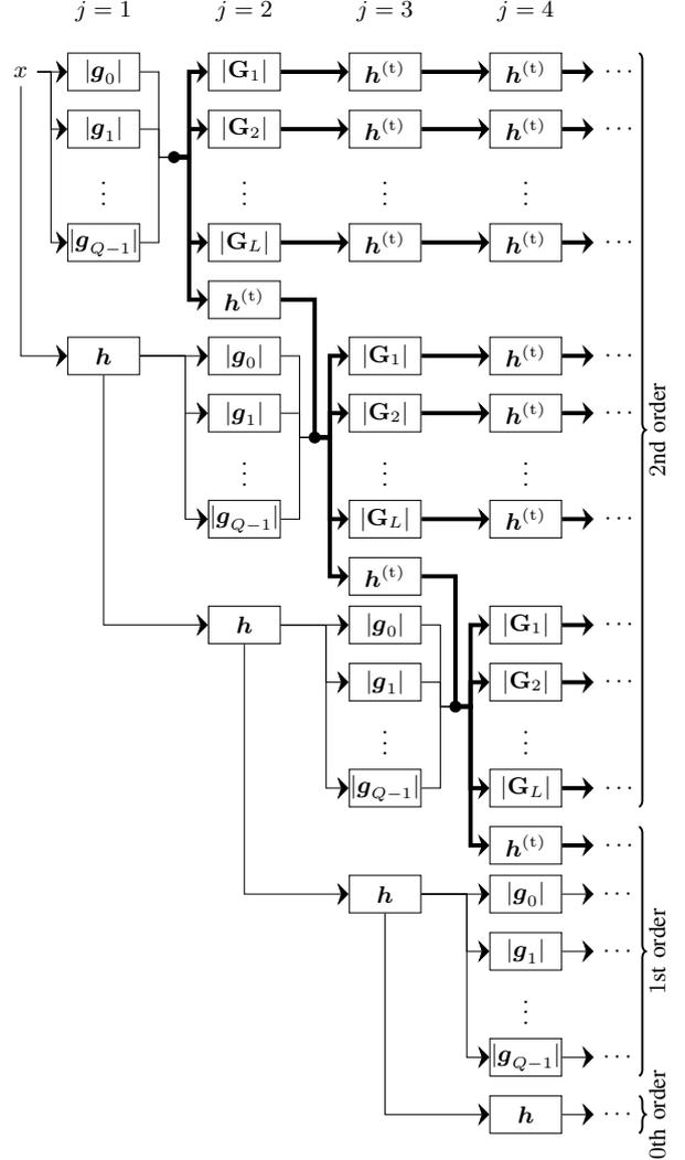
Fig. 8: A joint time-frequency scattering network. Each  $|g_k|$  block convolves a one-dimensional signal with the band-pass filter  $g_k$  and outputs its modulus. The outputs are aggregated into two-dimensional arrays shown by thick lines. A  $|G_\ell|$  block convolves a two-dimensional array with the band-pass filter  $G_\ell$  and outputs its modulus. The  $h$  and  $h^{(t)}$  blocks convolve only in time. All blocks subsample their output in time by 2.
