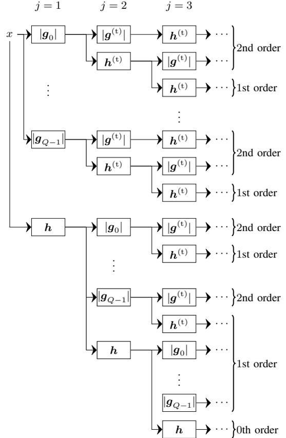
Fig. 5: A time scattering network. Each block with  $|g_k|$  or  $|g^{(t)}|$  outputs the modulus of the input convolved with a band-pass filter, subsampled by 2. Blocks with  $h$  and  $h^{(t)}$  convolve the input with a low-pass filter and subsample by 2.
