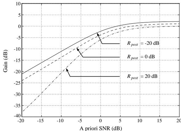
Figure 2: EMSR gain versus a priori SNR, for different values of the a posteriori SNR; topmost curve:  $\mathcal{R}_{post}(p, \omega_k) = -20$  dB; middle curve:  $\mathcal{R}_{post}(p, \omega_k) = 0$  dB; bottom curve:  $\mathcal{R}_{post}(p, \omega_k) = 20$  dB.
