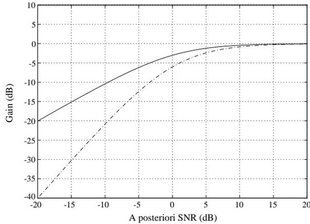
Figure 1: Gain versus a posteriori signal-to-noise ratio; solid line: Power subtraction; dashed line: Wiener.
