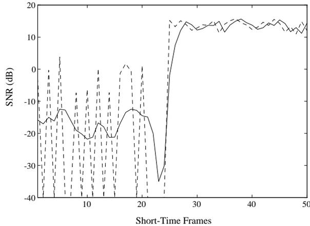
Figure 3: Signal-to-noise ratios in successive short-time frames; dashed curve: A posteriori SNR; solid curve: A priori SNR. For the first 25 short-time frames, the analyzed signal contains only noise at the displayed frequency, for the next 25 frames, a component with 15 dB SNR emerges at the displayed frequency. Parameter  $\alpha$  is set to 0.98.
