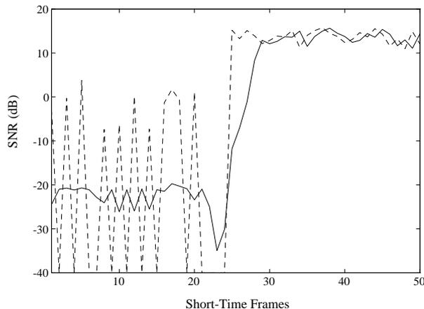
Figure 4: Signal-to-noise ratios in successive short-time frames; dashed curve: A posteriori SNR; solid curve: A priori SNR. The analyzed signal is the same as in Fig. 3. Parameter  $\alpha$  is set to 0.998.
