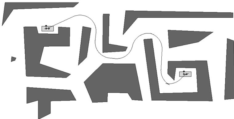
**Fig. 12.** A planned path for a car-like robot: the workspace is modeled by a grid of  $250 \times 150$  pixels; the total running of the algorithm is 2 seconds on an Indy Silicon Graphics.
