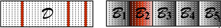
Fig. 1. Left: Traditional overcomplete dictionary. Each column represents an atom in the dictionary. Non-linear estimation has the full degree of freedom to select any combination of atoms (marked by the columns in red). Right: The underlying structured sparse piecewise linear dictionary of the proposed approach. The dictionary is composed of a family of PCA bases whose atoms are pre-ordered by their associated eigenvalues. For each image patch, an optimal linear estimator is calculated in each PCA basis and the best linear estimate among the bases is selected (marked by the basis in red).
