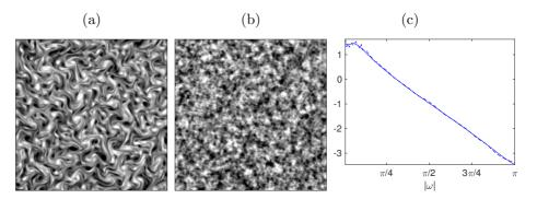
Figure 3: (a): Realization of a stationary turbulent vorticity field X. (b): Realization of a Gaussian maximum entropy model  $\widetilde{X}$  calculated from wavelet covariances estimated on a foveal graph. (c): The full line and dashed lines are the logarithms of the power spectrum of X and of the power spectrum of  $\widetilde{X}$  respectively as a function of the radial frequency  $|\omega|$ .
