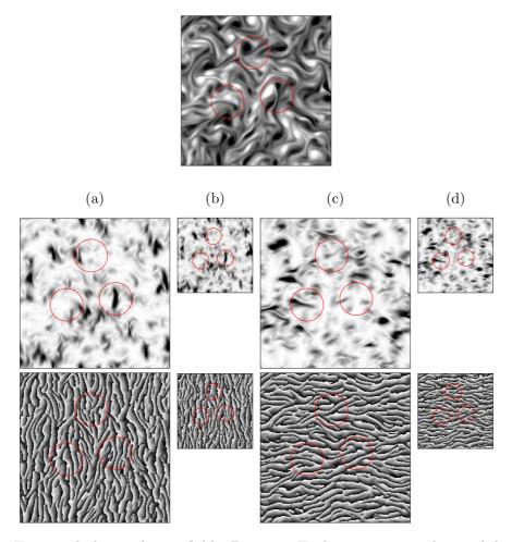
Figure 2: Top: turbulent velocity field. Bottom: Each image gives the modulus (above) or the phase (below) of wavelet coefficients  $x \star \psi_{\lambda}(u)$  for different frequency channels  $\lambda = 2^{-j}r_{-\ell}\xi$ . Large modulus coefficients are shown in black. The columns correspond to different scales and angles  $(j,\ell)$ . (a):  $(j,\ell)=(1,0)$ . (b):  $(j,\ell)=(2,0)$ . (c):  $(j,\ell)=(1,L/4)$ . (d):  $(j,\ell)=(2,L/4)$ .
