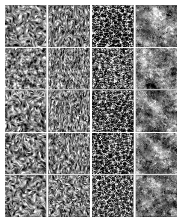
Figure 5: The first row shows a realization  $\bar{x}$  of X. The second to fifth row give realizations of microcanonical models A, B, C, D computed from  $\bar{x}$ . Each column corresponds to a different X. First column: Isotropic turbulent vorticity field. Second column: Non-isotropic turbulent vorticity field. Third column: Bubbles. Fourth column: Multifractal Random Walk.
