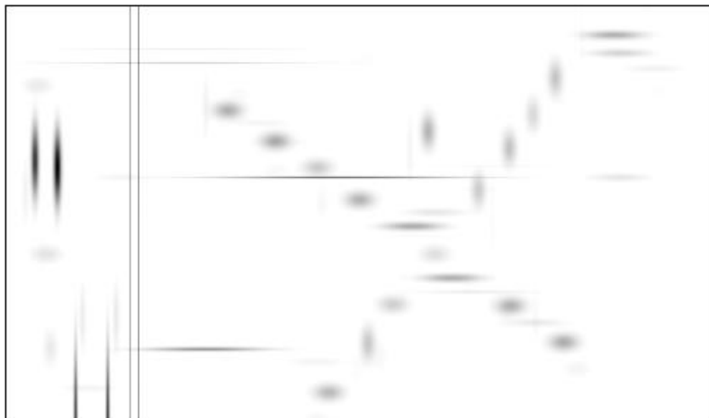
Figure 1(b): Time-frequency energy distribution Ef(t, \omega) of the signal shown in (a). The horizontal axis is time. The vertical axis is frequency. The highest frequencies are on the top. The darkness of this time-frequency image increases with the value Ef(t, \omega) .
