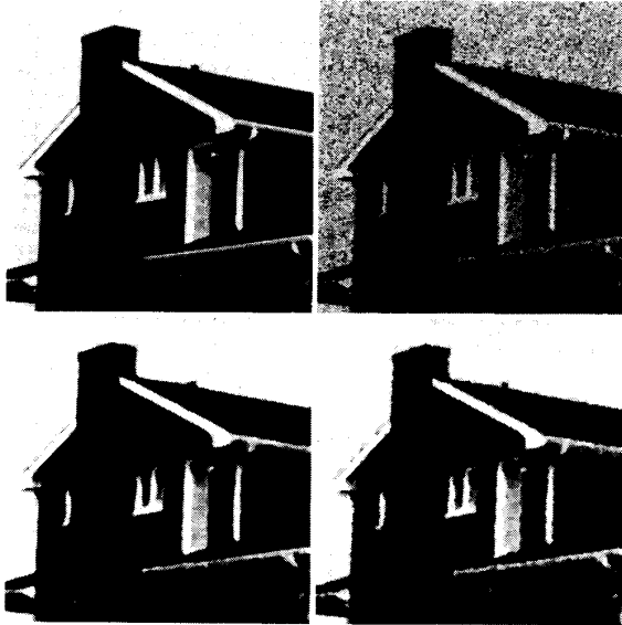
Fig. 14. Top left: original image. Top right: image contaminated by a Gaussian white noise. SNR is 2.9 db. Lower left: image reconstructed from the regularized maxima shown in the second column of Fig. 15. SNR is 14.3 db. Lower right: image reconstructed from the same modulus maxima, but without regularization along the maxima curves. SNR is 14.2 db.
