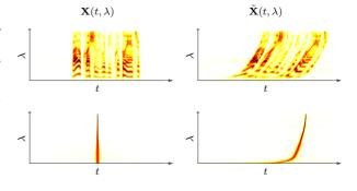
Fig. 6: Effect of frequency-dependent time-shifts  $\tau(\lambda)$  on scalograms of a speech recording (top) and a Dirac delta function (bottom). The two columns correspond to the original signal  $\boldsymbol{x}(t)$  and the transformed signal  $\tilde{\boldsymbol{x}}(t)$ , respectively.
