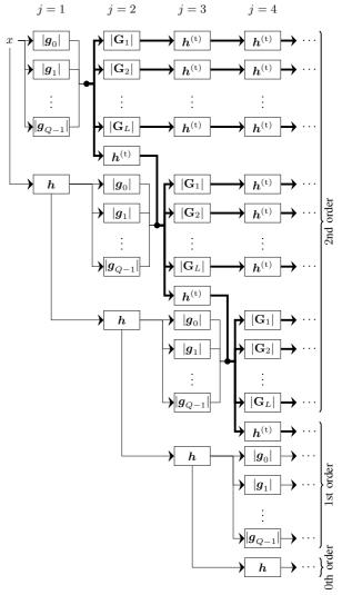
Fig. 8: A joint time-frequency scattering network. Each  $|g_k|$  block convolves a one-dimensional signal with the band-pass filter  $g_k$  and outputs its modulus. The outputs are aggregated into two-dimensional arrays shown by thick lines. A  $|\mathbf{G}_{\ell}|$  block convolves a two-dimensional array with the band-pass filter  $\mathbf{G}_{\ell}$  and outputs its modulus. The h and  $h^{(t)}$  blocks convolve only in time. All blocks subsample their output in time by 2.
