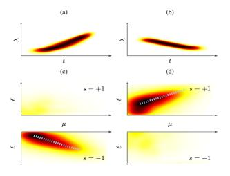
Fig. 9: Scalograms of two exponential chirps with chirp rates (a)  $\alpha = 4$  and (b)  $\alpha = -2$ . (c, d) Corresponding second-order joint time-frequency scattering coefficients  $\mathbf{S}_2 \boldsymbol{x}(t, \lambda, \mu, \ell, s)$ for fixed t and  $\lambda$ . The dotted lines satisfy  $s2^{\mu-\ell} = -\alpha$ .
