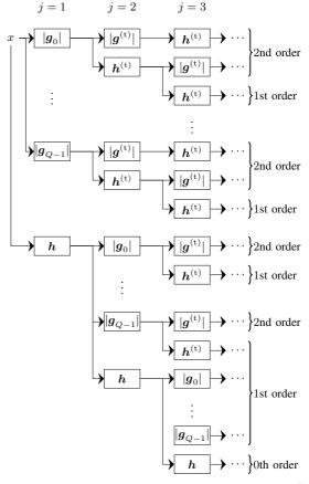
Fig. 5: A time scattering network. Each block with  $|g_k|$  or  $|g^{(t)}|$  outputs the modulus of the input convolved with a bandpass filter, subsampled by 2. Blocks with h and  $h^{(t)}$  convolves the input with a low-pass filter and subsample by 2.
