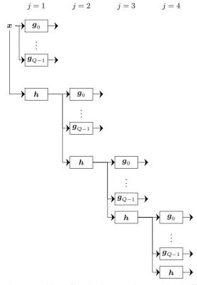
Fig. 3: Multirate filter bank computing wavelet coefficients for J = 4. Each block corresponds to a filter convolution subsampled by 2 where a boxed h is a low-pass filter and a boxed  $g_k$  is a band-pass filter. The depth corresponds to the octave index j while k = 0, ..., Q - 1 is the suboctave index.
