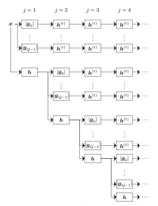
Fig. 4: Mel-spectrogram implemented as a convolutional network. Each  $|g_k|$  block convolves by a band-pass filter  $g_k[n]$ , computes the modulus, and subsamples by 2. Blocks containing h or  $h^{(t)}$  convolve by a low-pass filter and subsample by 2.
