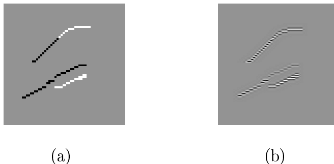
FIG. 11 – (a) : Examples of orthogonal grouplets. (b) : Orthogonal grouping bandlets corresponding to the grouplets in (a).
