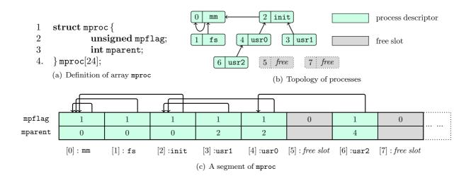
Figure 1: Minix 1.1 Memory Management Process Table (MMPT) structure
