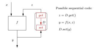
Fig. 4 The get/set principle breaks feedback loops
