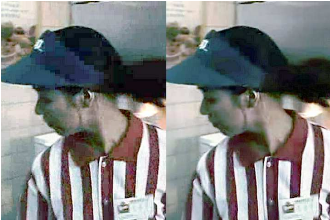
FIG. 16 – Left : Decompressed film frame corrupted by mosquito noise and blocking artifacts. Right : Distortion removal with bandlet thresholding.
