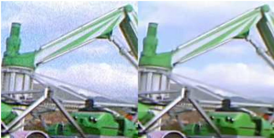
FIG. 15 – Left : Upconverted frame computed from an interlaced video corrupted by a camera noise. Right : Upconversion including a bandlet thresholding for noise removal.
