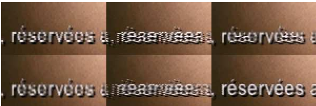
FIG. 8 – Deinterlaced zoom on lower left of Figure 5. Upper left : line doubling. Lower left : spatial interpolation. Upper middle : time weaving. Lower middle : time interpolation. Upper right : motion adaptive. Lower right : Let It Wave's deinterlacing.
