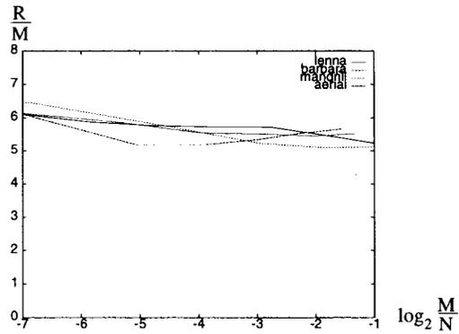
Fig. 13. Variations of  $R/M$  for an embedded wavelet coding of the test images.
