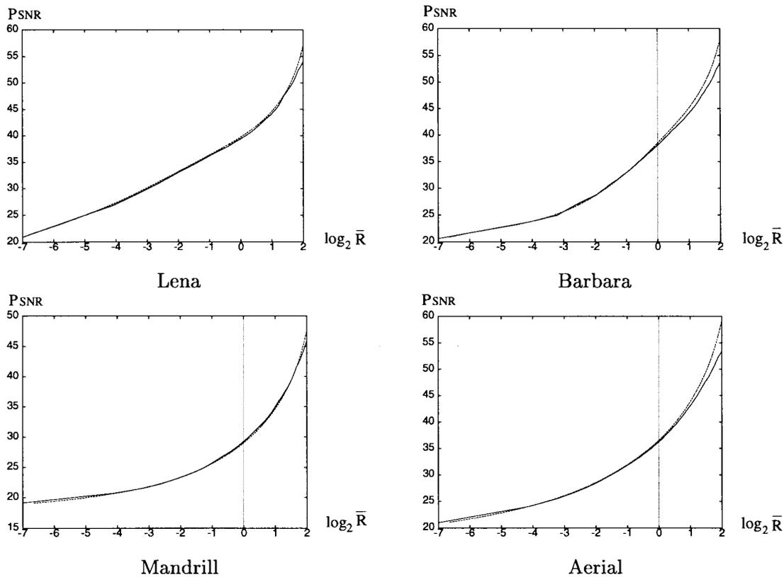
Fig. 14.  $P_{\text{SNR}}(D)$  (solid line) and  $P_{\text{SNR}}(\hat{D})$  (dashed line) for an embedded wavelet coding, with  $\hat{D} = (1 + \frac{1}{12})D_0(\bar{R}/5.5)$ .
