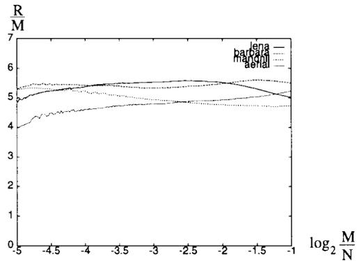
Fig. 10. Variations of  $R/M$  for the JPEG coding of the test images.
