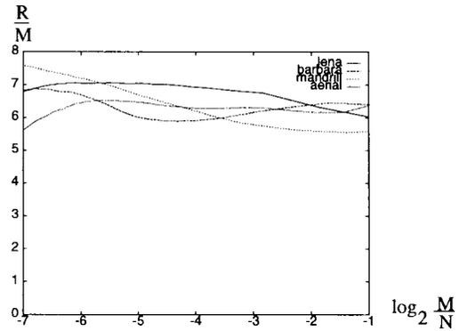
Fig. 7. Variations of  $R/M$  for the wavelet transform coding of the test images.
