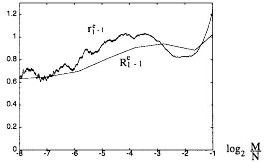
Fig. 12. Comparison of  $(R_1^e/M) - 1$  with the theoretical estimate  $r_1^e - 1 = 1/(2^{1/\gamma_M} - 1)$  for the embedded coding of Lena.
