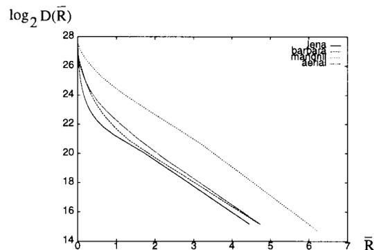
Fig. 2. Log distortion rate curve for the wavelet transform coding of each test image.
