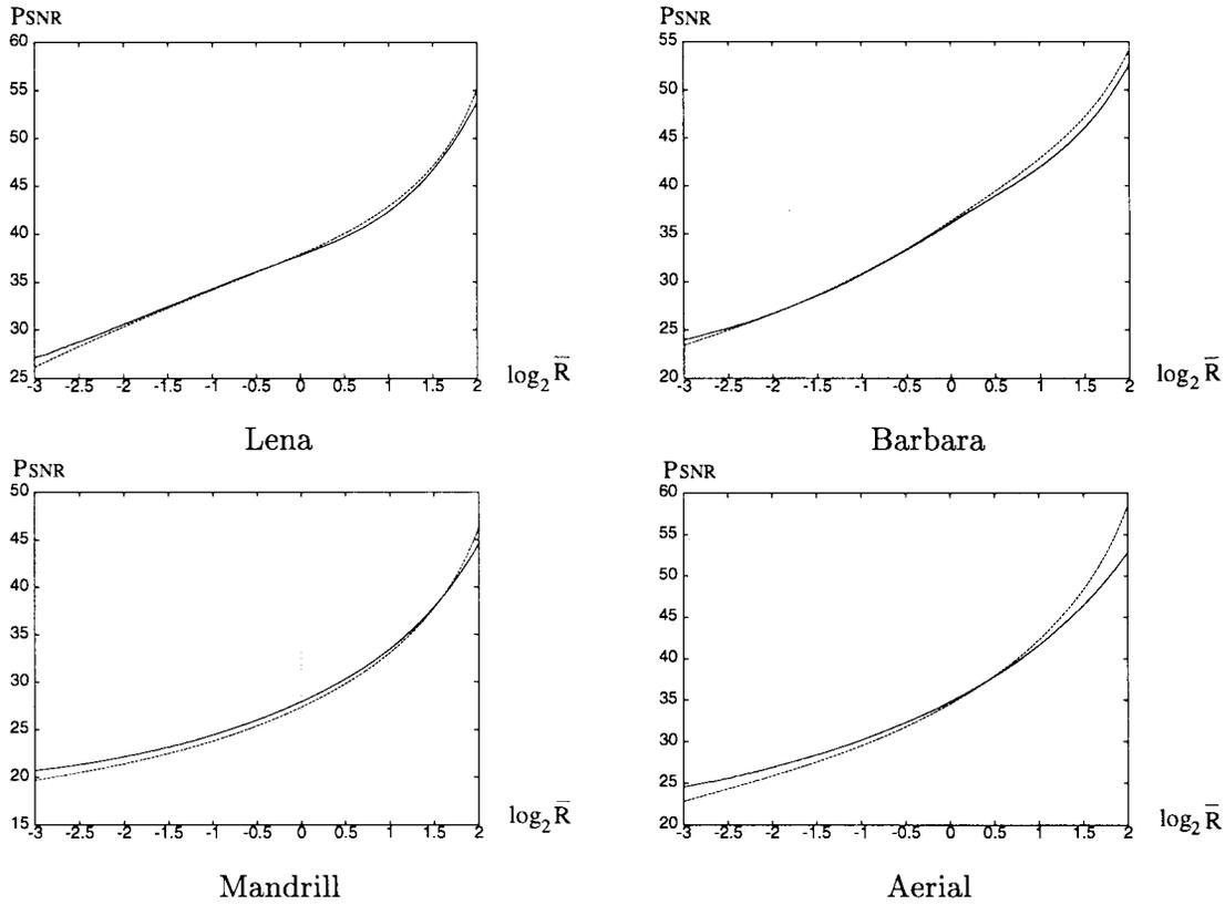
Fig. 11.  $P_{\text{SNR}}(D)$  (solid line) and  $P_{\text{SNR}}(\hat{D})$  (dashed line) for JPEG, with  $\hat{D} = (1 + \frac{1}{2})D_0(\bar{R}/5.5)$ .
