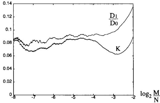
Fig. 5. Comparison of  $D_1/D_0$  with the theoretical estimate  $K = (2\gamma_M - 1)/12\theta^2$  for the wavelet coding of Lena.
