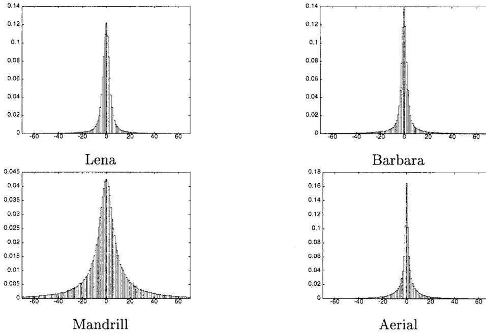
Fig. 3. Normalized histograms of the cubic-spline wavelet coefficients of the test images.
