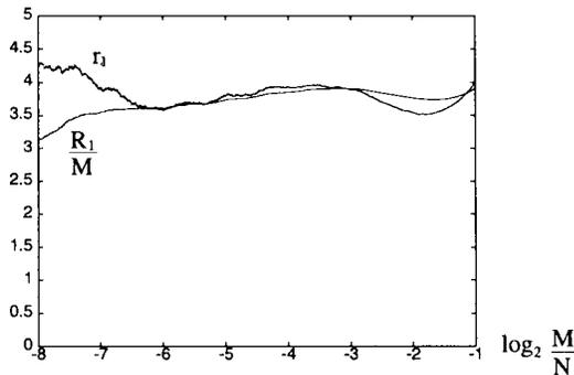
Fig. 6. Comparison of  $R_1/M$  with the theoretical estimate  $r_1 = 1 + (1 + \gamma_M)\log_2 e + \log_2 \gamma_M + \log_2 \theta$  for the wavelet coding of Lena.
