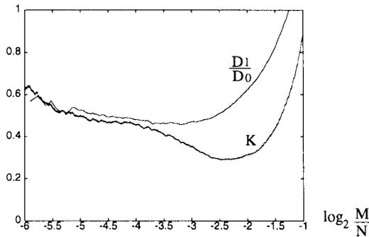
Fig. 9. Comparison of  $D_1/D_0$  with the theoretical estimate  $K = (2\gamma_M - 1)/12\theta^2$  for the JPEG coding of Lena.
