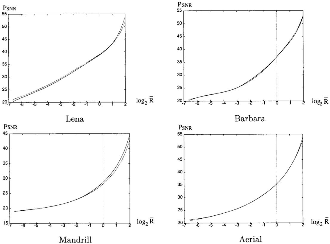
Fig. 8.  $PSNR(D)$  (solid line) and  $PSNR(\hat{D})$  (dashed line) for a wavelet coder with  $\hat{D} = (1 + \frac{1}{12})D_0(\bar{R}/6.5)$ .
