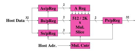
We have programmed both PAMs into long multipliers (n = 512) bits for  $P_0$ , and n = 2K bits for  $P_1$ ) computing  $P = A \times B + S$ , with A a n-bits multiplier, and B, S arbitrary size multiplicands and summands (see [10], [2])
