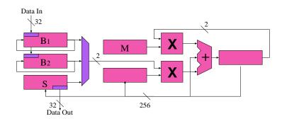
M. Shand recently ported this RSA system to a single  $P_1$  board; at 40 MHz, this design provides either two independent 600 Kb/s RSA encryption channels for 480b keys, or one 175 Kb/s RSA encryption channel for 970b
