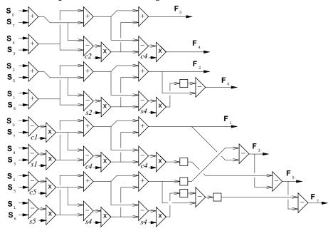
The overall design computes 48 fixed-point (32 bits outputs) operations (add, subtract, multiply and shift) on each 40 ns cycle, for a total of 1.4 Gops. To match this performance through software would require a 15 Gips processor.
