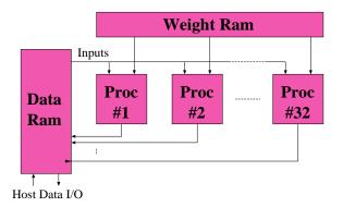
The latest realization, on  $P_1$ , can solve problems with up to 1400 variables, using 16-bit weights, for a total computing power of 500 megasynapses per second (the megasynapse is the traditional unit used in this field, it amounts to one million additions and multiplications, or one million terms of (2)).
