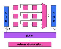
The convolver runs at 25 MHz, generating one pixel each 40 ns; it completes a single convolution pass over one  $512 \times 512$  image in 10 milliseconds;
