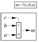
Note that:  $?(c, b, a) = (c \land b) \lor (\neg c \land a) = \text{if } c$  then b else a. Together with  $0 = {}_2(0)$ , the electrical ground and  $-1 = {}_2(1)$ , the electrical power supply whose bits are one at all times, the multiplexor provides a *basis* for boolean algebra:  $\neg b = ?(b, 0, -1), a \lor b = ?(a, a, b)$  and  $a \land b = ?(a, b, a)$ .
