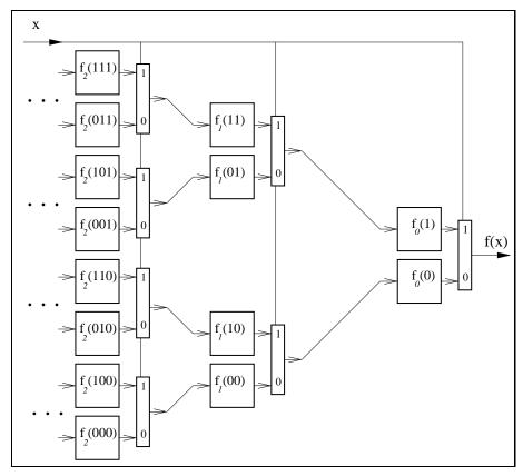
In this schema, each rectangle denotes a multiplexor with control input x (label 1 on the high input, 0 on low); each square denotes a register: with initial value 0 when the label inside is zero, one otherwise (example 1).
