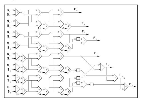
Consider an arbitrary synchronous network, such as the one drawn above which computes the fast discrete cosine transform for appropriate coefficients  $s_1, \dots, s_7, c_1, \dots, c_7 \in \mathbb{N}$ . How can we pipe-line a sequence of finite precision integer computations through such a network? By simply adjoining a (synchronous) *reset* input, and replacing each register equation  $r = 2 \times i$  in the network by the register with reset:
