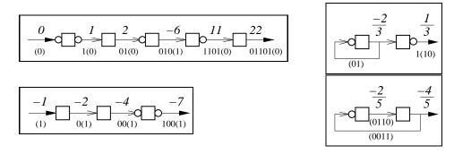
In our schemas: circles denote inverters and squares denote registers with initial value *zero*. A register with inverters on both sides (example 1) is recognized as having initial value *one*: it computes 1 + 2x.
