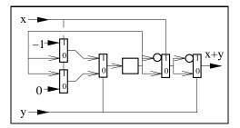
While it is by nature an *infinite* process, algorithm SDD(f) generates a finite synchronous circuit (in finite time) if and only if function f may be defined by some *finite automaton*:
