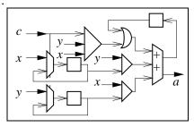
This design leads to more economical circuits than the Atrubin (see [K81]) or the Chen and Willoner constructions [CW79]. From here on, a circle with an  $\times$ inside denotes this serial-serial multiplier.
