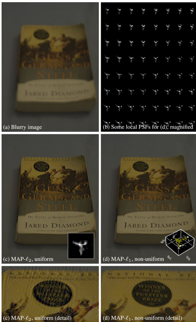
Fig. 7 Blind deblurring of real camera shake, example 2. The result of blind deblurring on a real camera shake image (a), captured with a shutter speed of 1 second, using the MAP approach of Cho and Lee with both the uniform and non-uniform blur models. Also shown in (b) are some of the local PSFs generated from the blur kernel in (d) at various points in the image. In the blurry image, most of the text on the book cover is too blurred to read. Deblurring the image with the uniform blur model (c) allows some of the text on the cover of the book to be read, however, after deblurring with our non-uniform model (d), all but the smallest text becomes legible. The blur kernel in (d) covers \pm 0.4^\circ in \theta_x and \theta_y , and \pm 0.9^\circ in \theta_z
