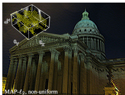
Fig. 9 Poor performance of MAP- \ell_2 with non-uniform blur model. The corresponding blurry image can be seen in Fig. 6. Shown is the estimated kernel and deblurred result when using our non-uniform blur model in the algorithm of Cho and Lee with \ell_2 regularization on the kernel. As can be seen, the \ell_2 regularization is not sufficient to produce a good estimate of the kernel, and results in a deblurred output containing many artifacts
