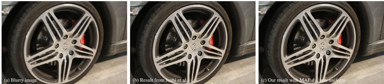
Fig. 11 Blind deblurring of an image from Joshi et al. (2010). A handheld image with camera shake (a), from Joshi et al. (2010), with the deblurred results from the original work (b) and using the MAP- \ell_1 method with our blur model (c). We obtain a comparable result, with-
