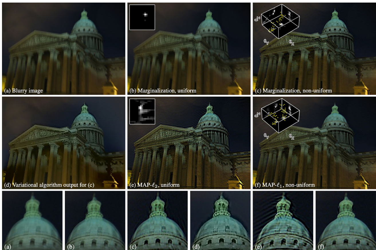
Fig. 6 Blind deblurring of real camera shake, example 3. A hand-held image with camera shake (a), captured with a shutter speed of 1 second, with the results of blind deblurring using the marginalization algorithm of Fergus et al. under both a uniform (b) and non-uniform (c–d) blur model, and the MAP algorithm of Cho and Lee with a uniform (e) and non-uniform (f) blur model. The variational output (d) is estimated using the marginalization algorithm for the non-uniform case (calculated
