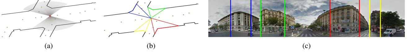
Figure 2: Overview of data generation from Google Street View images and cadastre maps. We first (a) cast 30m rays to the sides of each Street View capture location at 1^\circ intervals, then (b) compute intersections with facades and select the widest view, and (c) project onto the panoramas and crop and warp the facade images according to Street View metadata.
