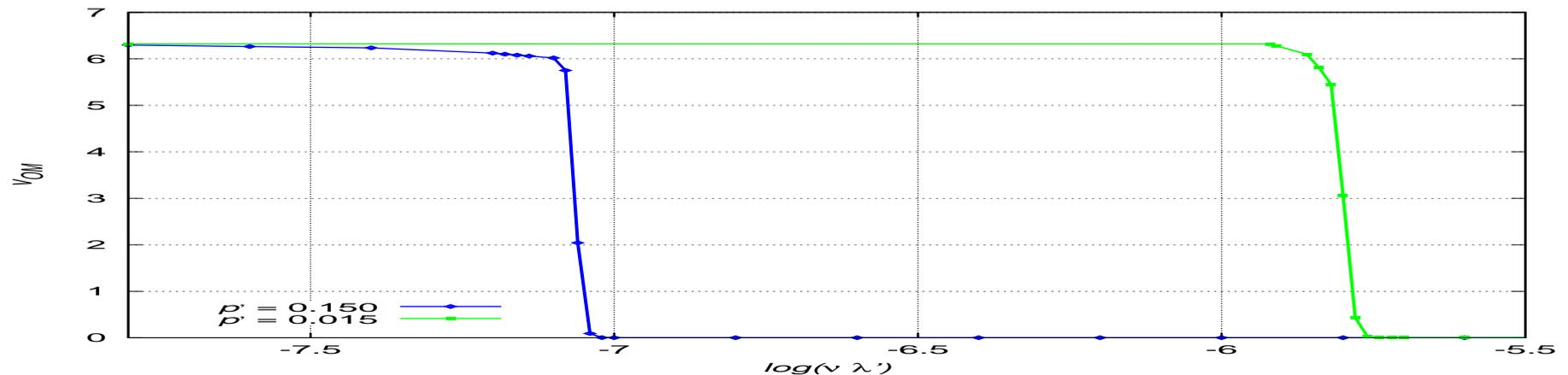
Mean speed on a given distance  $0M$  in function of the density of interferers  $\mu = \lambda' \nu$ .
