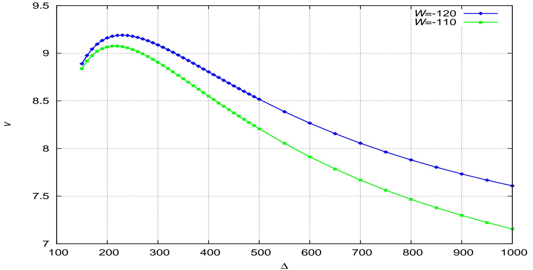
Note the optimal inter-relay distance  $\Delta$ .
