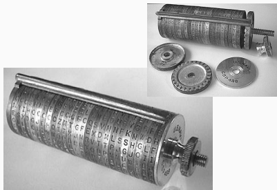
Wheel – M 94 (CSP 488) Poly-alphabetical Substitution
