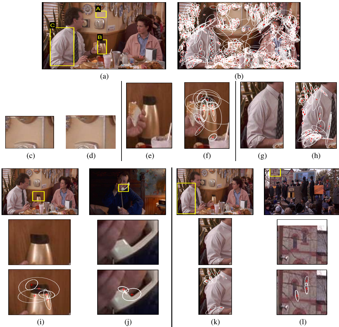
Fig. 15. Examples of challenging object searches. (a) Keyframe from the movie ‘Groundhog Day’ with three query regions (denoted A,B,C). (b) The same keyframe with affine covariant regions superimposed. (c,e,g) Query region close-ups. (d,f,h) Query close-ups with affine covariant regions superimposed. (i-l) Example retrievals for object B (i-j) and object C (k-l). Each column shows (top) a keyframe from the retrieved shot with the identified region of interest, (middle) a close-up of the image, and (bottom) a close-up of the image with matched affine regions superimposed. Query analysis: Query A (plain wall) does not contain any visual words and hence returns no results. Query B (coffee pot) retrieves two shots taken from very similar viewpoints (the 2nd ranked is shown in (i)). Other shots are not retrieved as affine regions extracted on the object either include background or cover specular reflections, which change with viewpoint and lighting conditions. The first false positive (ranked 3rd) is shown in (j). Query C (the white shirt) retrieves three correct shots (the 2nd ranked is shown in (k)) but most of the matches are on the background object. This is because affine regions on the shirt are detected on creases, which change as the person moves. The first false positive (ranked 4th) is shown in (l).
