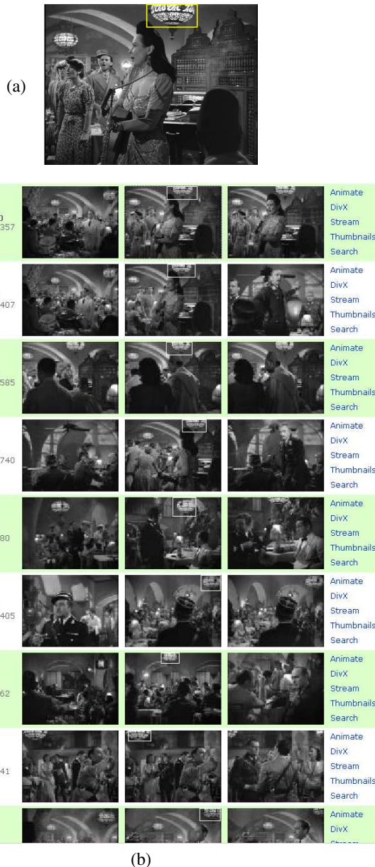
Fig. 7. Object query example III: Casablanca. (a) Keyframe with user specified query region (lamp). (b) Screenshot showing the first eight ranked shots. Each shot is displayed by three thumbnails showing (from left to right) the first frame, the matched keyframe with the identified region of interest shown in white, and the last frame of the shot.
