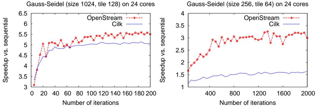
Fig. 19. Speedups obtained on smaller resolutions of Gauss-Seidel, highlighting the advantages of OpenStream point-to-point synchronization.
