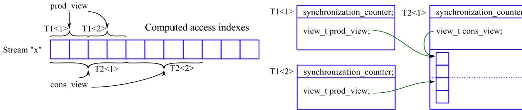
Fig. 15. Matching producers with consumers in a stream for an example of two streaming tasks (top) communicating through stream “x”, conceptually represented as an infinite sequence of indexed data elements and the resulting frame chaining (bottom). This illustrates the `stream_match_views` function in Figure 17.
