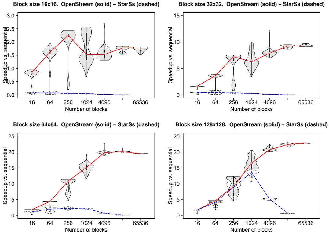
Fig. 22. Sparse LU factorization for 4 different configurations, speedup vs. sequential.
