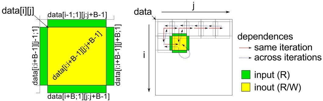
Fig. 12. Data dependencies, within one single iteration, for the Gauss-Seidel application in Figure 11.
