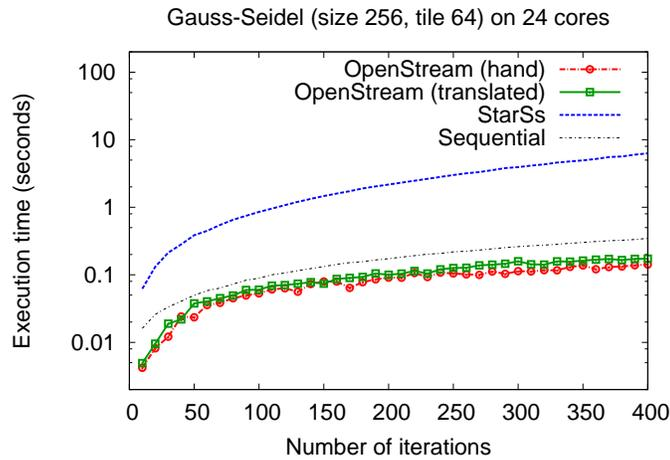
Fig. 21. Task-level scalability of OpenStream and StarSs. For a  $B \times B$  tiles matrix and  $I$  iterations, the number of tasks is  $I * B^2$ , here spanning from 640 (10 iterations) to 25600 (400 iterations) tasks.
