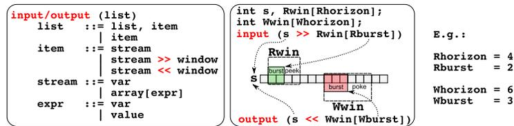
Fig. 1. Syntax for input and output clauses (left) and illustration of stream access through windows (right).
