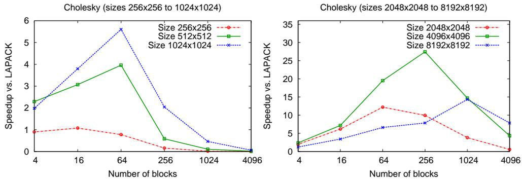
Fig. 23. Cholesky factorization speedups of OpenStream vs. LAPACK.
