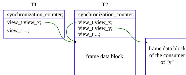
Fig. 14. Data structures used for generating data-flow code: simple example of streaming tasks (top) with the frame and view data structures (middle) and frame layout and chaining (bottom).
