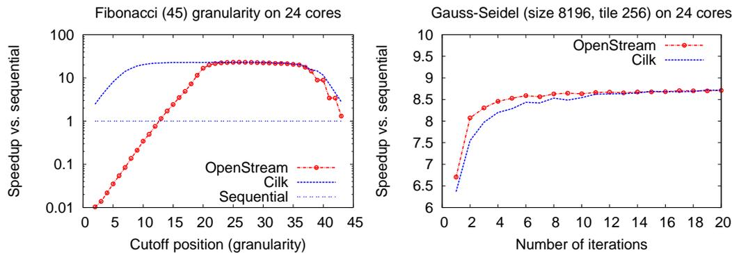
Fig. 18. Performance comparison with Cilk on Fibonacci (left) and Gauss-Seidel (right).
