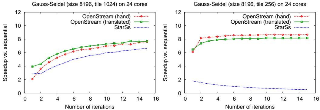
Fig. 20. Gauss-Seidel performance comparison with StarSs and our translation of StarSs to OpenStream. The optimal tile size for StarSs is  $1024 \times 1024$  (left) and  $256 \times 256$  for OpenStream (right).
