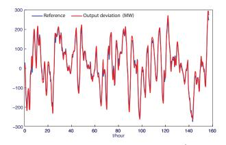
PI control:  $\zeta_t = 19e_t + 1.4e_t^I$ ,  $e_t = r_t - y_t$  and  $e_t^I = \sum_{k=0}^t e_k$ Each pool pump turns on/off with probability depending on 1) its internal state, and 2) the BPA reg signal
