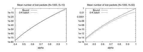
Fig. 3. Exact values and for the mean number of lost packets for "0-K" batch compared to the bound
